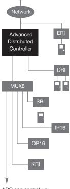
ADC can control up to 32 Sub-controllers (with restrictions)
