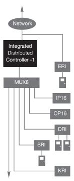
IDC-1 can control up to 16 Sub-Controllers (with restrictions)
